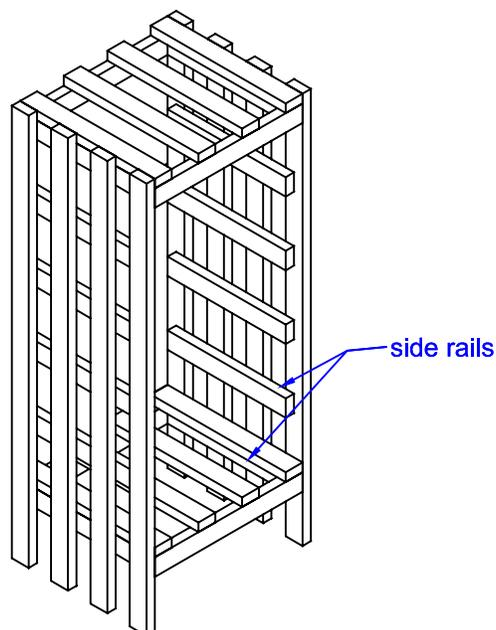
3. Keep adding shelves from the bottom up and nailing them on. Securing the top last.
