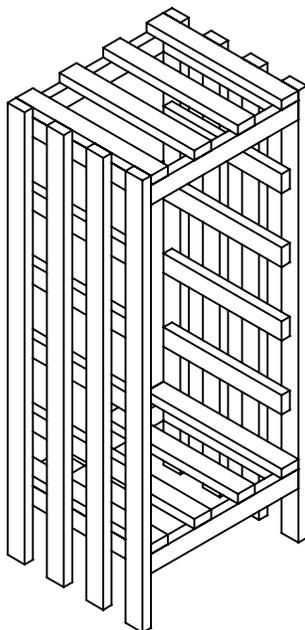
2. Nail only the bottom shelf to the side rail. Leave the top shelf to keep the spacing.
